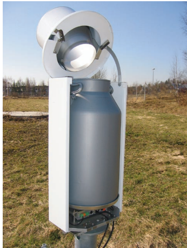
Fig. 2. The gauge with enclosure opened.
