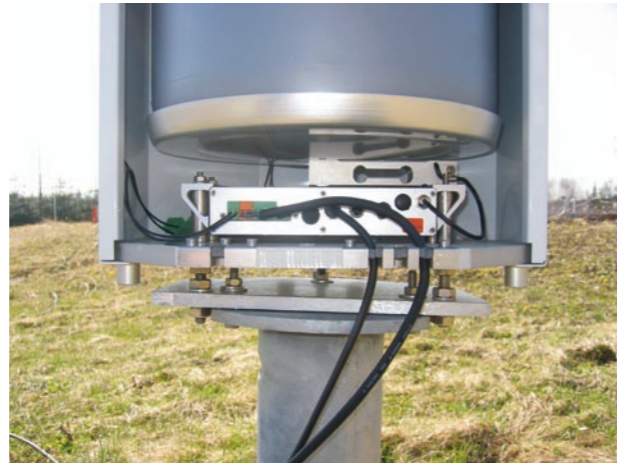
Fig. 3. Electronics unit and load cell are situated under the weighing platform.
