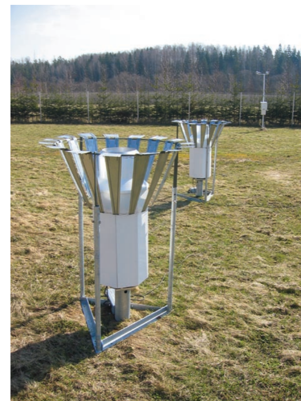
Fig. 1. Vaisala all weather precipitation gauge with wind shield.
