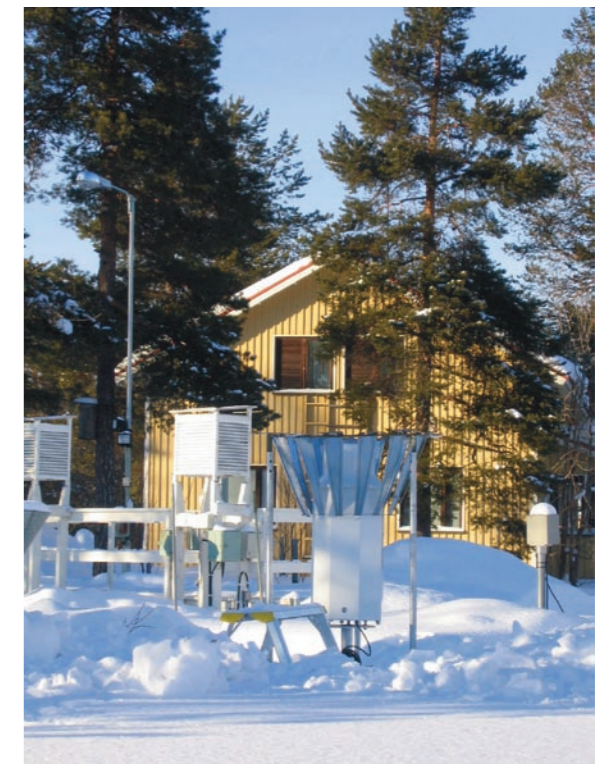
Fig. 6. The Vaisala gauge installed on the FMI Sodankylä test field.
