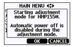
4. Press **OK** to move on to the adjustment and select the quantity you want to adjust. The list of quantities displayed in the figure below vary according to the configuration of your HMP155.
