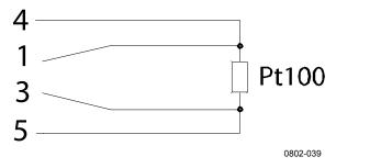
Figure 8 Pins Connected to Pt100 (passive output version)
