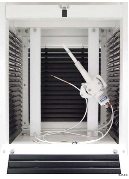
Figure 6 HMP155 with T-Probe Installed in Stevenson Screen
