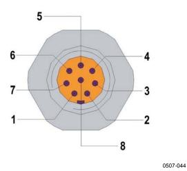
Figure 7 Wiring of HMP155 8-Pin Connector
