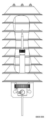
Figure 5 T-probe Installed in DTR502B
