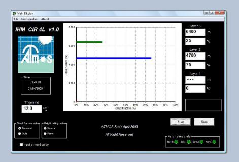
The software package process all data using a special algorithm designed by ATMOS, and provides numerical and graphic description of the cloud cover, in terms of cloud fraction and evaluation of cloud altitude height.
