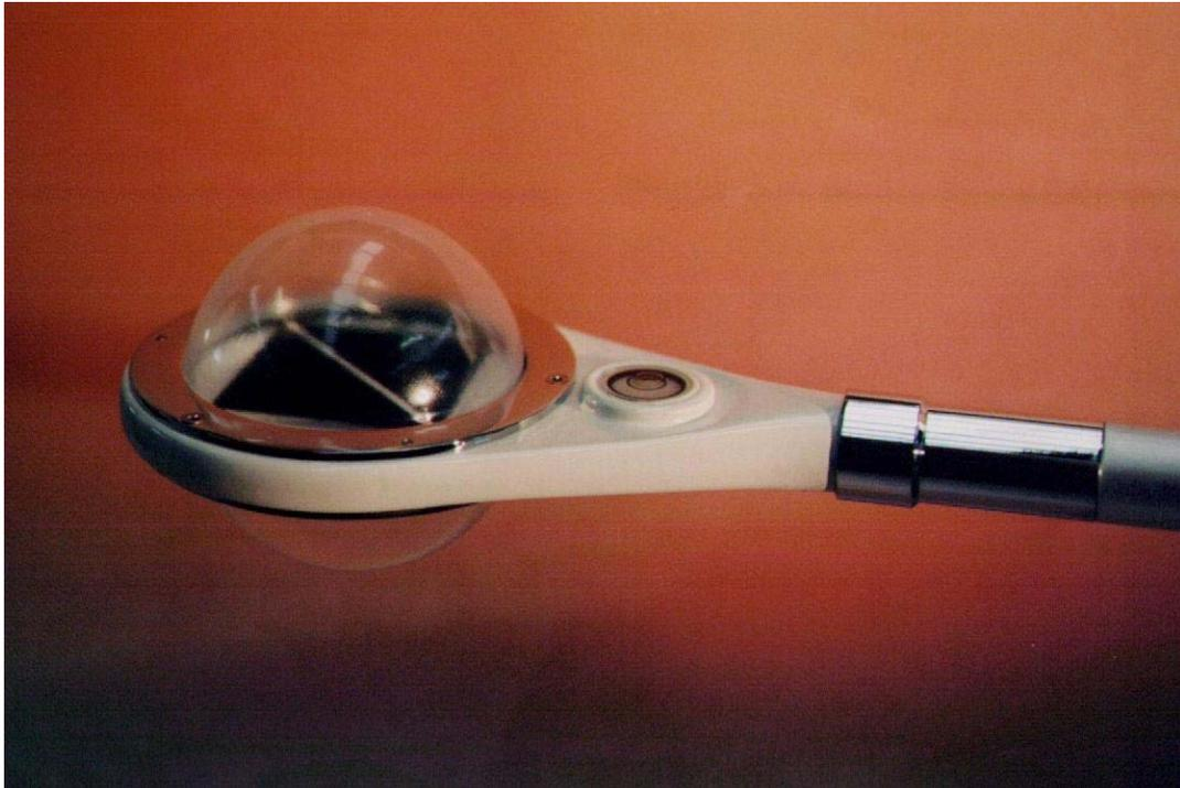
The Middleton CN1-R Net Pyrradiometer measures the net total radiation flux (solar, terrestrial, and atmospheric) downward and upward through a horizontal surface. It is suitable for solar energy studies in agriculture and meteorology.
