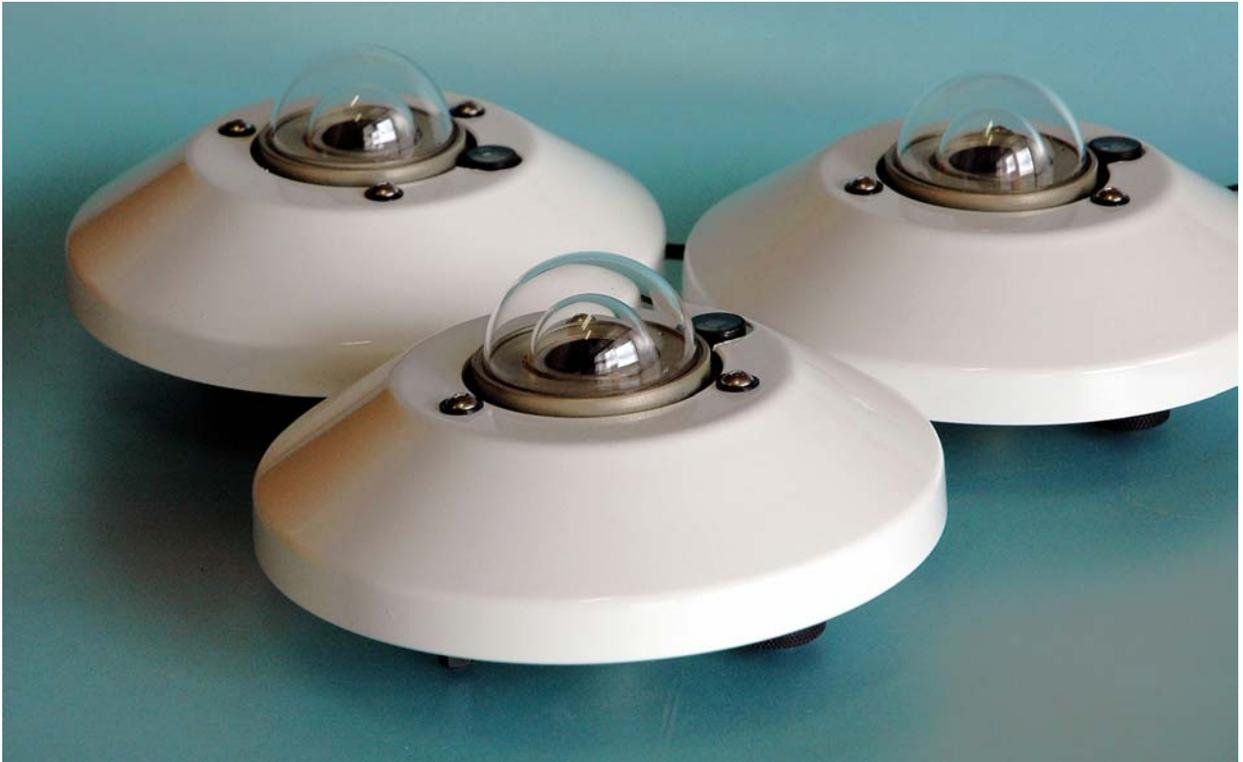
The Middleton EQ08-S is a precision pyranometer for the measurement of global solar irradiance on a plane surface. It exceeds the international accepted specifications for a high quality pyranometer. The EQ08-S incorporates a second generation precision thermoelectric sensor that has exceptionally low directional error without compromise to signal strength or response time. The EQ08-SE version has an in-built amplifier to give a millivolt output for easy signal measurement.
