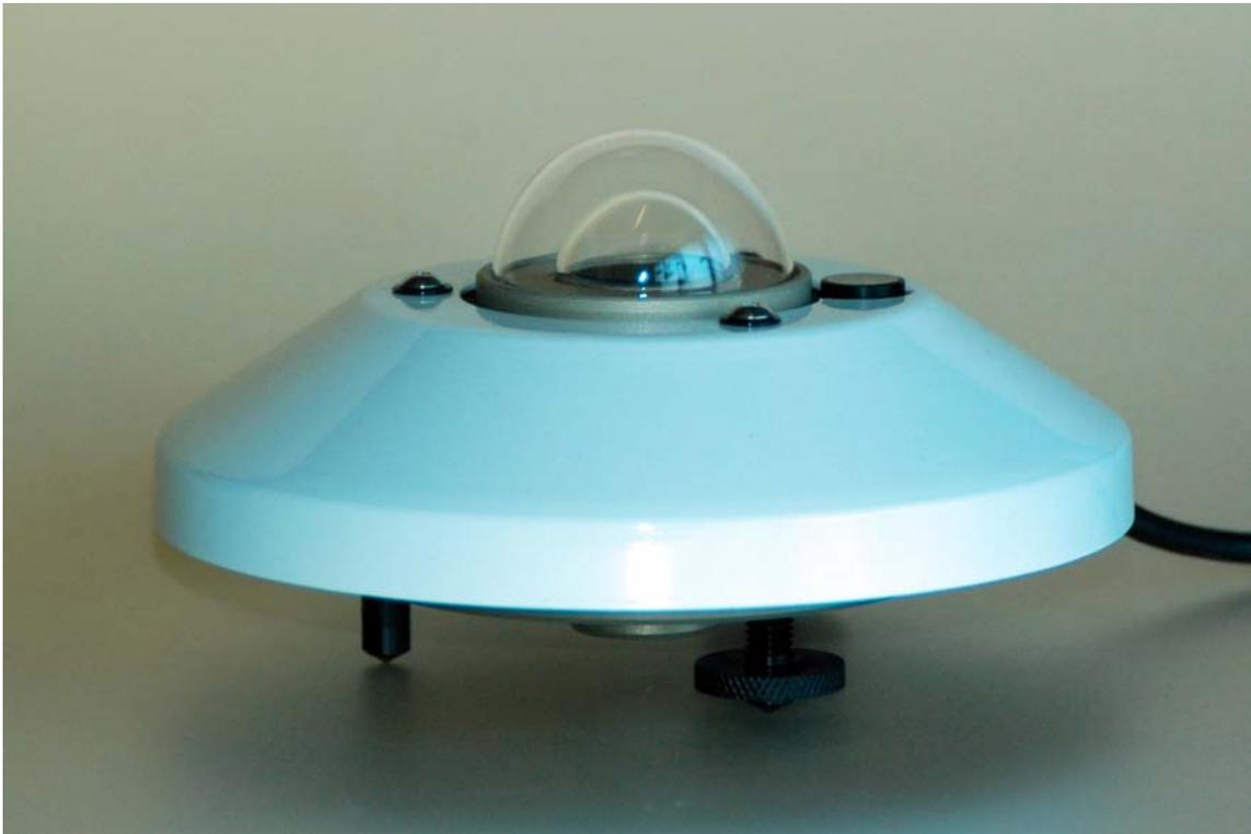
The Middleton EQ08 is a precision pyranometer for the measurement of global solar irradiance on a plane surface. It exceeds the international accepted specifications for a good quality pyranometer. The EQ08 incorporates a state-of-the-art precision thermoelectric sensor. The EQ08-E version has an inbuilt signal amplifier.
