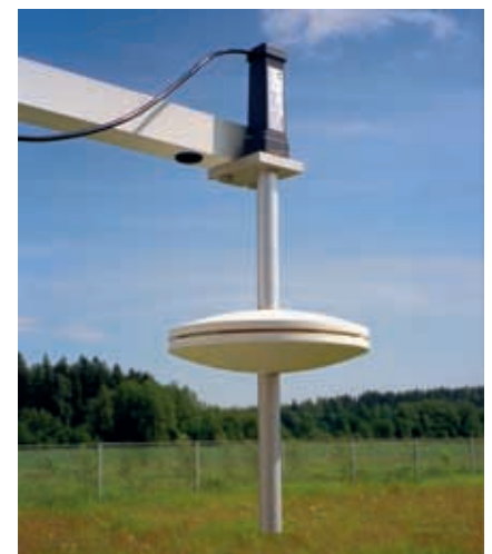
The PTU210 paired with the SPH10/20 Static Pressure Head.
