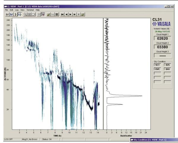
The cloud intensity is shown as a point graph, in which the colour is proportional to the strength of the return signal from the altitude in question. The backscatter profile is presented as a line graph in instant and average modes. Both modes can be displayed simultaneously.
