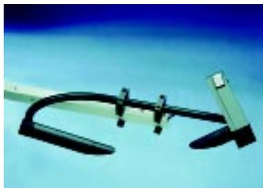
proportional to the amount of water on the capacitive sensing surfaces, while optical intensity is proportional to the volume of reflecting particles.
