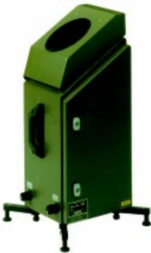
A special tilt sensor is provided as standard for automatically compensating uneven terrain. Installation is made easier and faster when no exact leveling is required. The cloud coverage algorithm in the CT25KAM is a further development of the algorithm specified by FAA. Cloud coverage (amount) is reported in 0 to 8 octas, according to WMO regulations.
