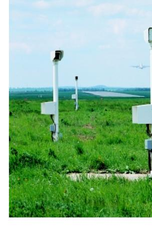
One background luminance meter, mounted on top of the light transmitter, is sufficient per runway to measure the background luminance value needed in visibility calculation.
