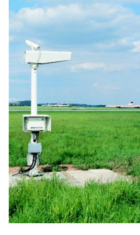
lying on estimates of projected light power, every transmitted pulse is measured. Atmospheric transmittance is then calculated as the ratio of received and transmitted light power on a single pulse basis. Receiver electronics are gated to receive only light pulses from the transmitter, and will not accept any interference light during the interval.
