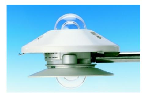
The CM7B and CM14 albedometers are suitable for measuring net global radiation and/or albedo over many differing types of surface. Both sensors are of equal sensitivity. They also have conical lower screens, to prevent illumination of the lower glass dome at sunrise and sunset.
