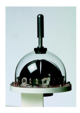
Rain drops and frosting on the outer dome have negligible effect upon the performance of the DSU12 sensor. The solar heating of the dome via the blackened element pairs and the restricted ventilation combine to assist in quickly melting snow deposits and frost. Heavy snow falls may reduce the effectiveness of operation.
