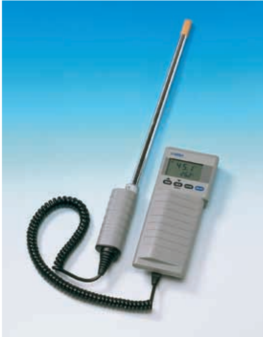
The HMI41 Indicator equipped with the HMI46 Probe is an ideal combination for spot checking and field calibration.
