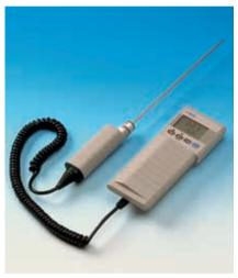
HMI41 with the HMP42 Probe.
