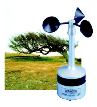
The WAA252 Heated Anemometer is an optimum choice for non-freezing applications. It offers the linearity and sensitivity of a welldesigned cup anemometer plus the advantage of heating carried out right where it is needed - in the cups. Foil heaters are included in each cup and in the cupwheel hub. For easy maintenance the cupwheel is removable, with a 2-pin connector for heating electricity.
