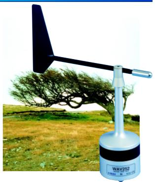
The WAV252 is normally used with the WAA252 Heated Anemometer. A single 24VDC (5.5A) power supply such as the Vaisala WHP25 is able to feed both devices simultaneously. The WAV252 can be mounted on Vaisala's regular WAC151 crossarm and its output interface is compatible with that of the regular WAV151 vane. Therefore, upgrada-tion to a heated-vane system is easy - just a minimal wiring alteration is needed in the crossarm's junction box.
