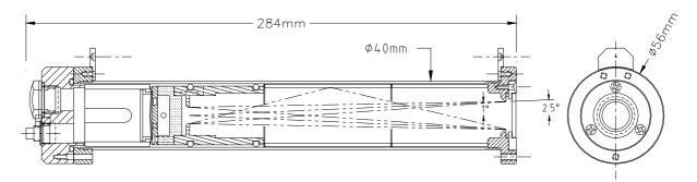
Black carbon nanotube (CNT) sensor surface has flat spectral response and excellent stability. Can be operated with all Middleton Solar Trackers: APT-02, AST-02, AST-03. Aiming diopter conveniently located on top of instrument. Temperature compensated sensor assembly is thermally isolated from the instrument body. Optical geometry, and baffling, is set by four precisely located apertures. Supplied with User Manual and Calibration Certificate.
