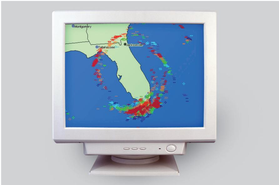
In discharge display mode, the individual lightning locations are shown as + or - for identifying positive or negative polarity and are color coded in time intervals. The marker size can be adjusted to represent the event's amplitude in kiloamps (kA).
