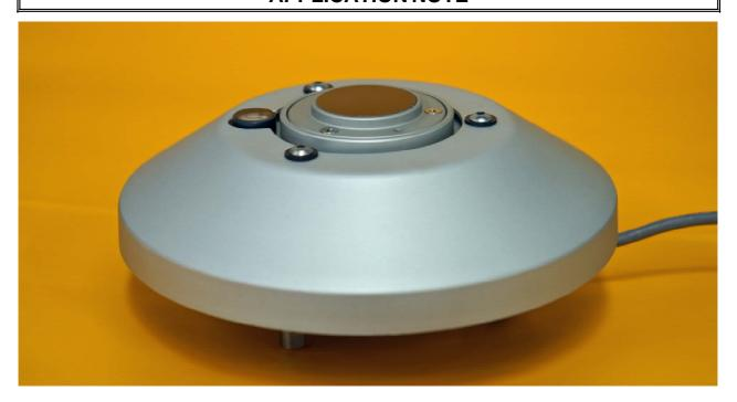
The Middleton Solar PG01 Pyrgeometer is for measuring long wave radiation emitted by the atmosphere (downwelling) or the Earth surface (upwelling). It uses a passive thermoelectric sensor shielded by a flat silicon window. The window is coated to exclude radiation below 4.5 µm. The PG01 is sealed and fully weatherproof.
