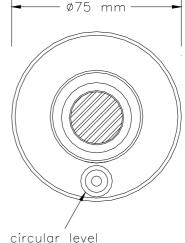
Meets the ISO 9060:2018 specifications for a Spectrally Flat Pyranometer of Class B, and the equivalent WMO specifications for a Good Quality Pyranometer. Temperature-compensated thermoelectric sensor.
