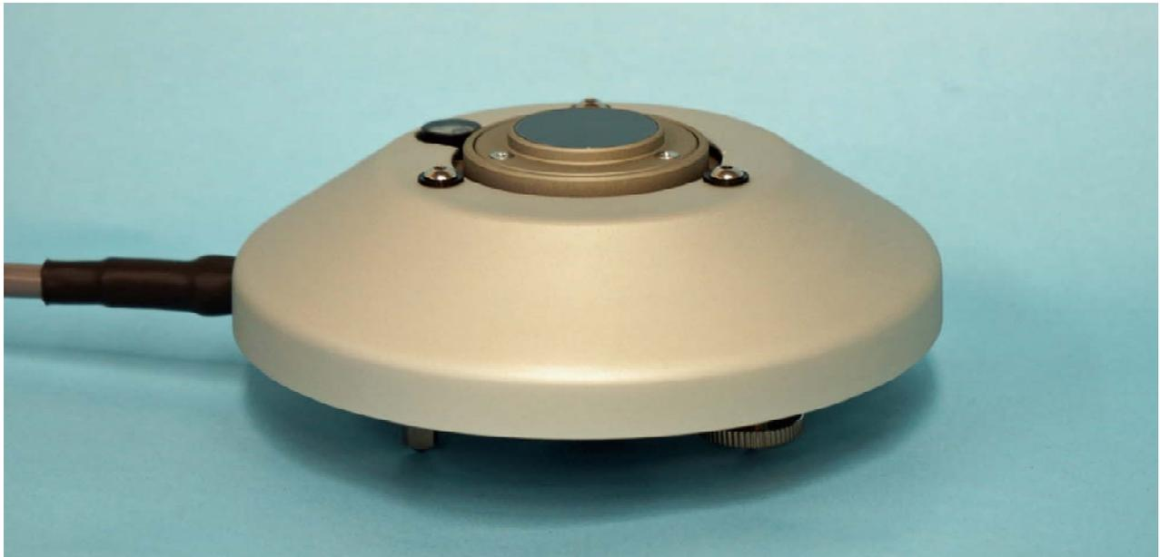
The Middleton Solar PG01-E Pyrgeometer is for measuring long wave radiation emitted by the atmosphere (downwelling) or the Earth surface (upwelling). It uses a passive thermoelectric sensor shielded by a flat silicon window. The window is coated to exclude radiation below 4.5  $\mu\text{m}$ . The PG01-E has in-built signal amplifier. It is sealed and fully weatherproof.
