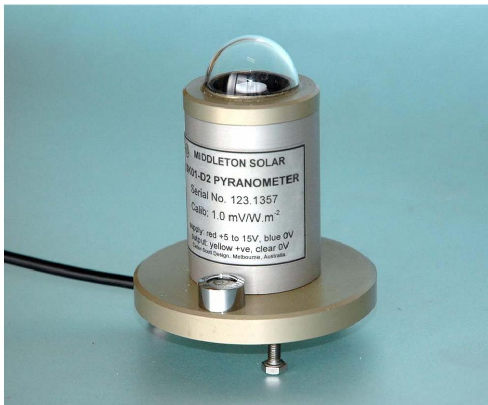
The SK01-D2 is a simple pyranometer for measuring total solar global radiation on a horizontal surface. The SK01-DP2 version incorporates a special filter to limit its sensitivity to the Photosynthetically Active Radiation region of the solar spectrum (400-700nm).
