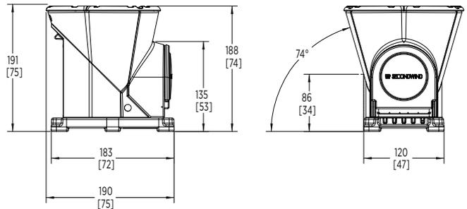
Dimensions in cm (inches), rounded to the nearest unit. Solar panels and mounting hardware not shown.
